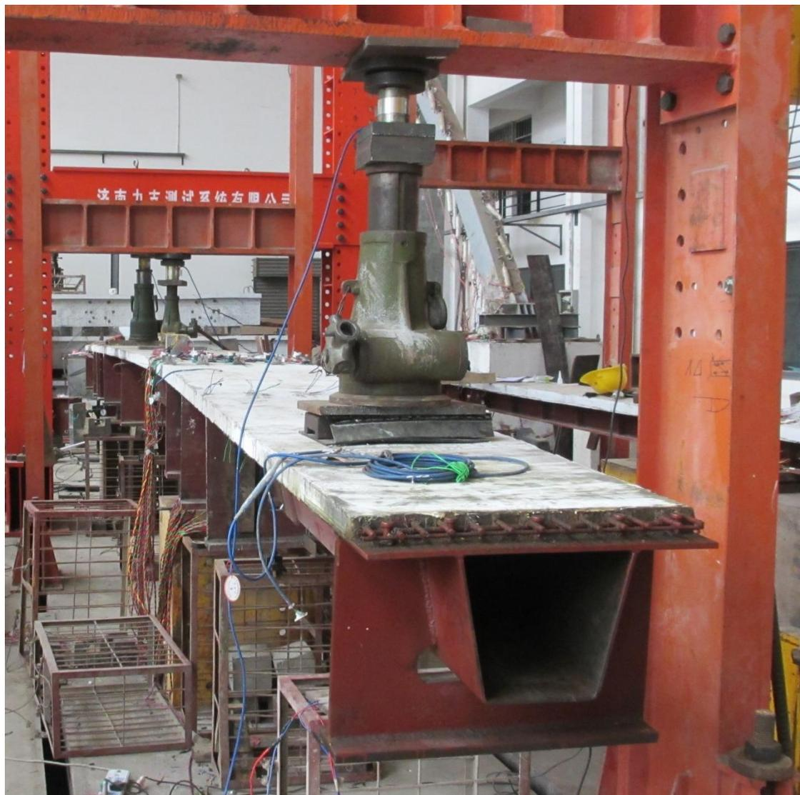
UHPC开裂前抗拉强度—42.7MPa
